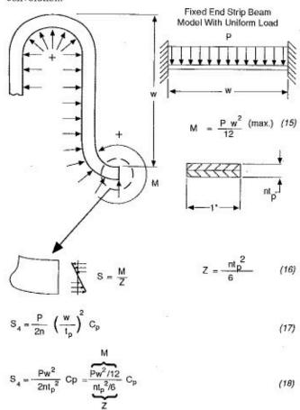
The calculated value of S4 is defined as a primary bending stress. As such, the sum of the primary membrane stress (S3) plus the primary bending stress (S4) must be less than the allowable limit. The limit is defined as the yield strength of the material in the as-installed condition or Cm times Sab. A wide ranging unpublished parametric study by the EJMA organization found that the average error between the calculated value of S3+S4 and FEA results was 2.8% with a maximum error of 8.2%.
