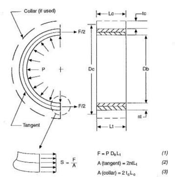
$$S_1 = \frac{P(D_b + nt)^2 L_1 E_b k}{2 (nt E_b L_1 (D_b + nt) + t_c k E_c L_c D_c)}$$
